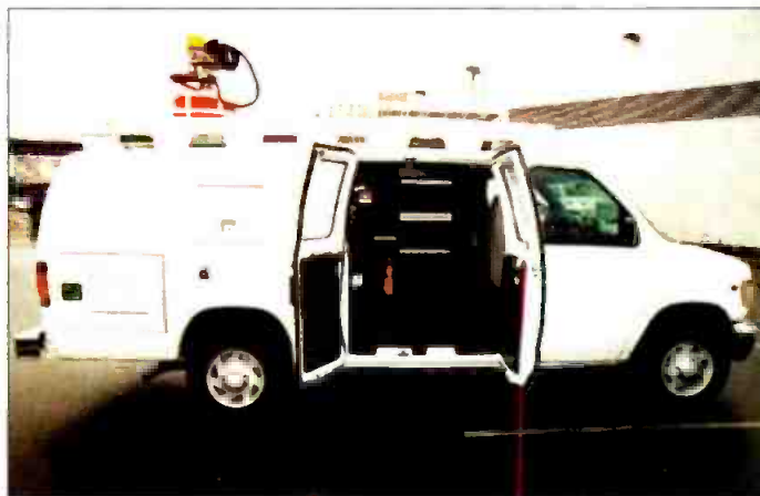
KOMO-DTV's field measurement van, constructed by Frontline Communications of Clearwater, Fla., will be used to perform reception tests on its DTV signal throughout the Seattle market.
