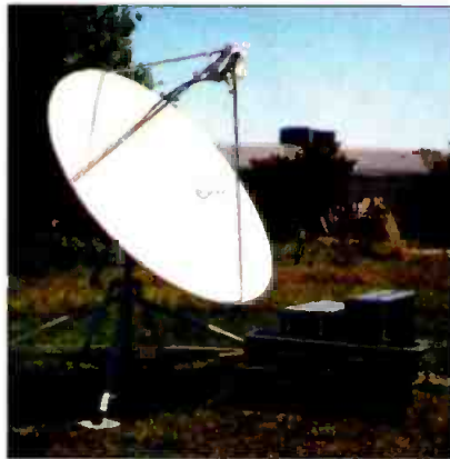
Comtech's new 2.4-meter flyaway unit can transmit in the C-, Ku- or X-band frequencies.
